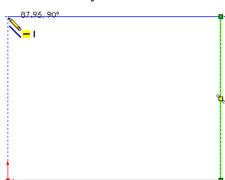
Finish the shape by drawing a vertical line and select the origin as the end point as shown.
